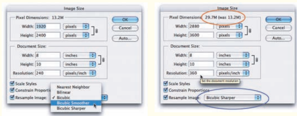
(Left) Photoshop's Image>Image Size dialog box before interpolating, and with Bicubic Smoother selected. (Right) The Image Size dialog box after upscaling by 50% (note the change in file size—circled in red).
